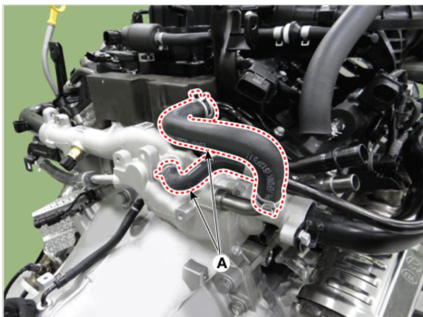
4. Disconnect the oil cooler hose B (A).
